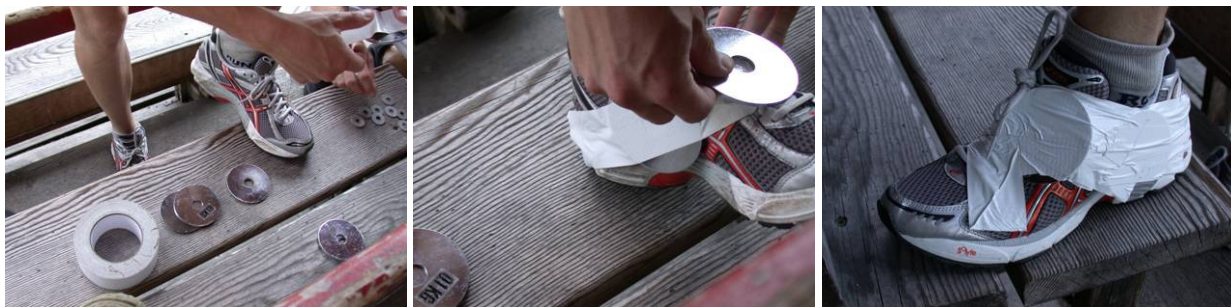
Figures 5-7: Weight equalization of MBT shoes and running shoes
